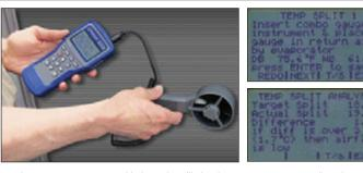
Just two measurements with the probe will give the target temperature split and actual temperature split across the evaporator and compare the two.
