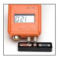
Note: When checking digital wood meter models with the MCS-1, the meter should be set to default: 4-pin, 70°F, Douglas Fir to obtain the nominal 12% and 22% readings. If set to 2-pin, 70°F, Douglas Fir, the readings will be 12.7%, and 23.6%.
