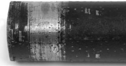
Figure 14B – 300 PD Chuck Marks in Prep Area
