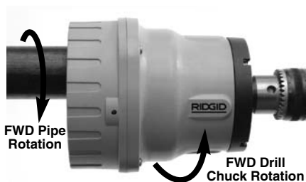
Figure 11 – Proper Use of Prep Tool to Remove Pipe OD Coating With Rotating Pipe
