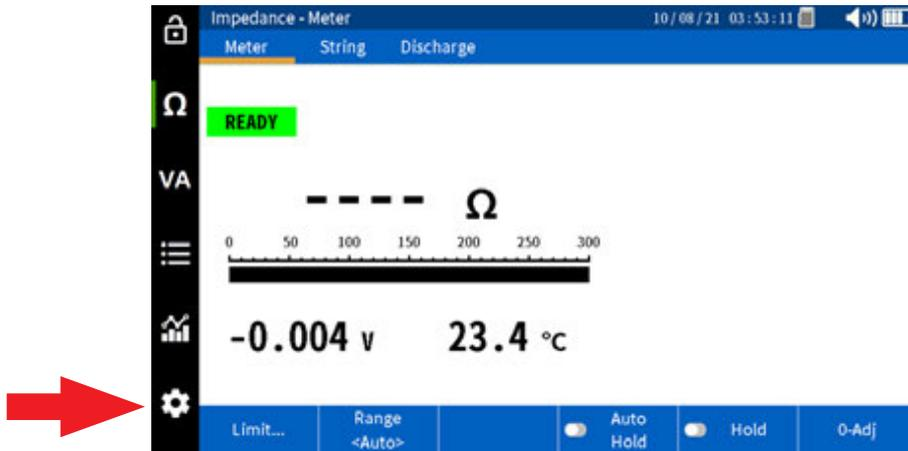
Under the impedance tab, the temperature measurement scale can be selected (Celsius or Fahrenheit). On the BITE5-SE model the display units can be set to either Ohms or Siemens. This will allow the measured values and displayed data to be viewed in either Ohms or Siemens.
