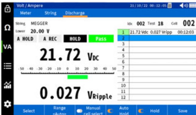
Take measurement of the each following cell. Each measurement shall be saved in sequence with a cell number, date and time stamp.
