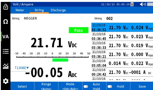
Press "Hold" to freeze the measurement on the screen.
