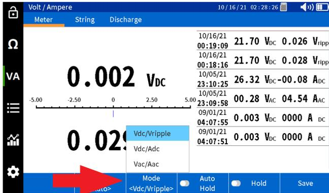
If using the CT set the correct range on the BITE5.
