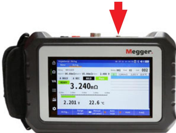
The displayed screen shall be saved to the SD card as a bitmap file.
