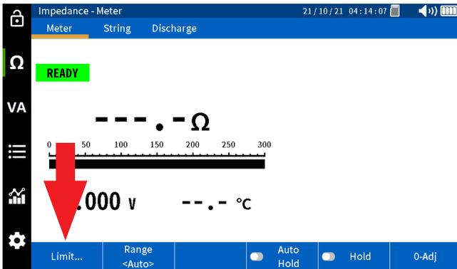
This screen will allow you to program a warning and alarm limit for the impedance value and a lower limit for the voltage. This is an optional step. Select OK when done.
