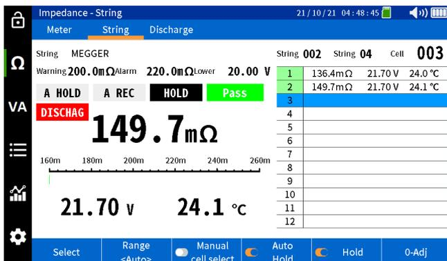
Continue taking a measurement of each cell in sequence on the string until you reach the last cell in the string.
