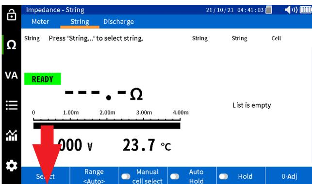
Select desired string. Select "New Test" to start a new test on the selected string.
