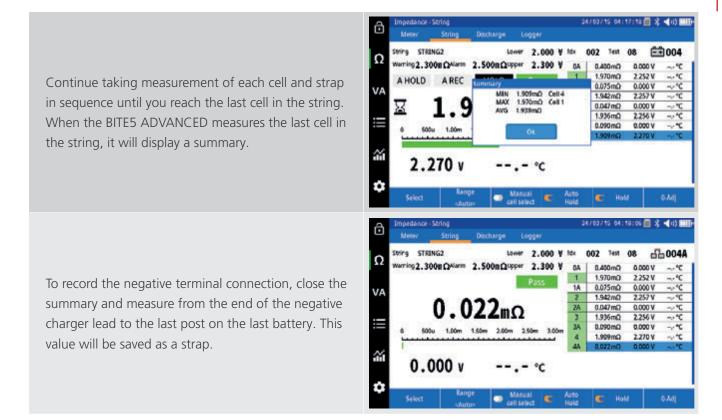
Performing an impedance test on a parallel battery string.
