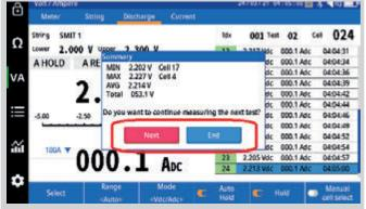
Performing an impedance and discharge test (special testing)
