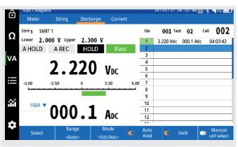
Take measurement of each following cell. Each measurement shall be saved in sequence with a cell number, date, and time stamp.
