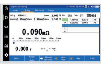
Continue taking measurements until the parallel string is reached. At this point move the AC CT to the path that was just measured and then continue measuring the cells and straps if the parallel string.
