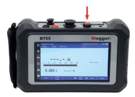
The displayed screen shall be saved to the SD card as a bitmap file. The bitmap will be located at the following path.
