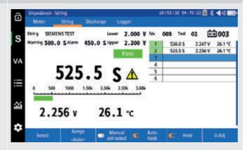
Continue taking measurement of each cell and strap in sequence until you reach the last cell in the string. When the BITE5 ADVANCED measures the last cell in the string, it will display a summary.
