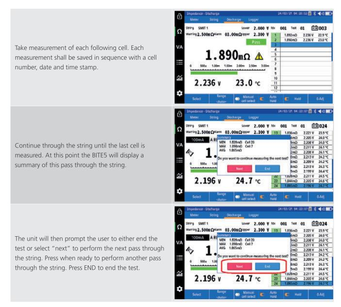
**NOTE**: This value will be associated with the internal impedance changes associated with sulfated plates. It may not correlate with other causes of cell aging such as plate corrosion.
