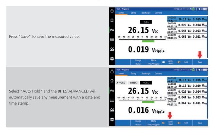
Adding a Ripple (AC) Voltage, Ripple (AC)Current or a Float (DC) Current value to a string.
