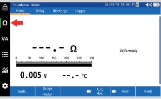
When the Ohm ( $\Omega$ ) ICON is selected the BITE5 Advanced will use the Duplex inputs.
