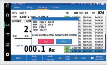
The unit will then prompt the user to either end the test or select "next" to perform the next pass through the string. Press when ready to perform another pass through the string. Press END to end the test.
