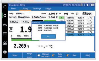
Performing a conductance test on a battery string.
