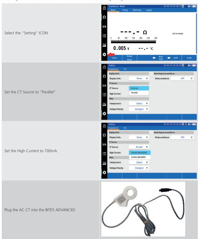
Place the AC Current clamps on the parallel path.
