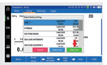
Start testing by placing the probes on the first cell. The unit will beep when the measurement is complete and save the measured values to memory. The results will be displayed on the screen.
