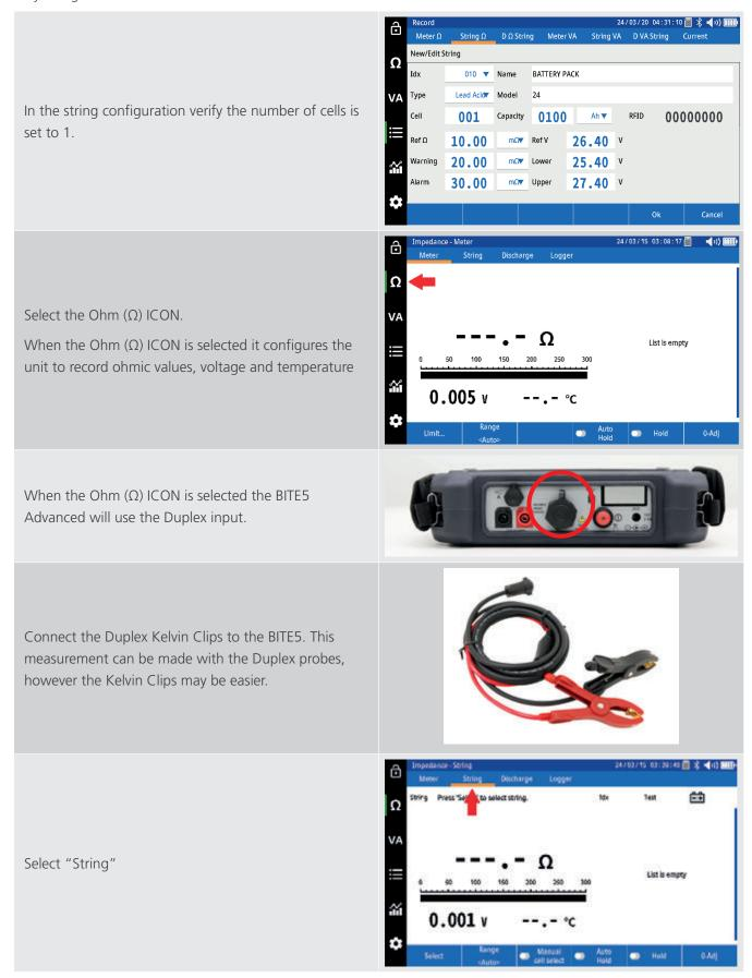
Performing an impedance test on a battery pack.
