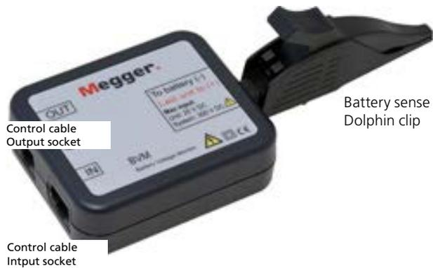
cell and each unit can handle up to 20 V. The BVMs connects to the batteries in a “daisy-chain” fashion, thereby providing easy and economical expandability to meet the testing requirements for small-to-large battery bank systems. Up to 120 BVMs can be daisy-chained in a single battery bank under test.
