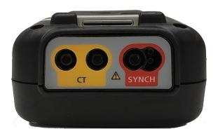
The current clamp plugs into the CT inputs. The sync cable will plug into the "SYNCH" input.
