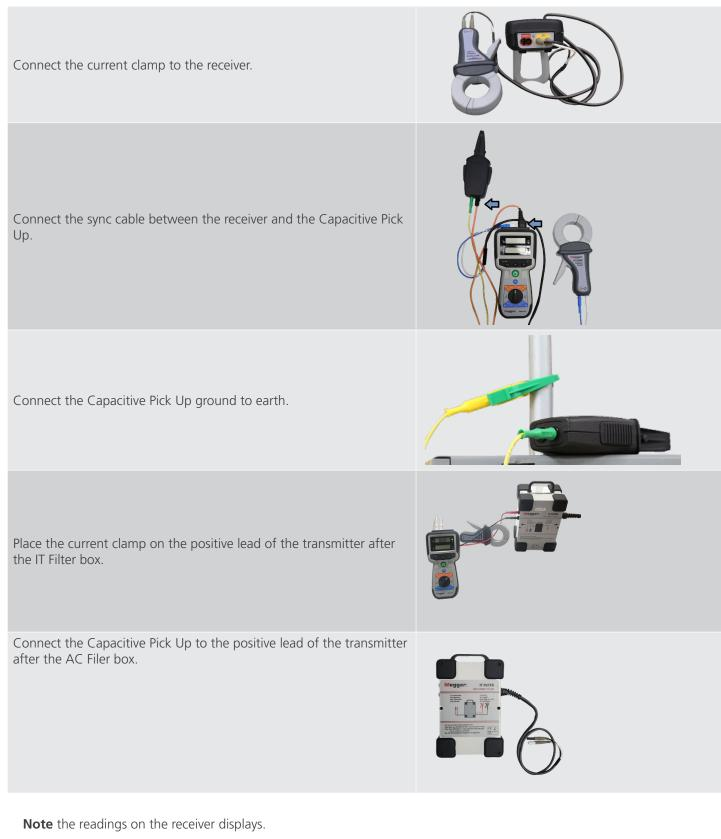
The top display will indicate the current the fault is drawing.
