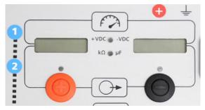
Once the transmitter had completed booting the lower left voltage display will be flashing.
