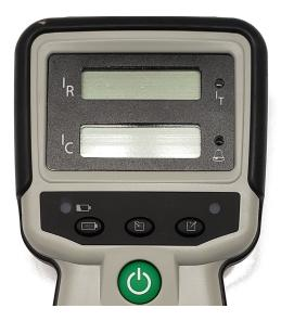
Set the alarm level on the receiver to 50%. This can be either a visual only alarm or a visual and audio alarm, depending on how it is set
