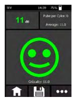
The user is also supported with the presentation of the measurement results. Measurement data is evaluated automatically, and feedback about the condition of the asset is provided visually by means of a smiley face and other ways. If the customer wishes other trending limits for the interpretation of the data, this can simply be individually customized.
