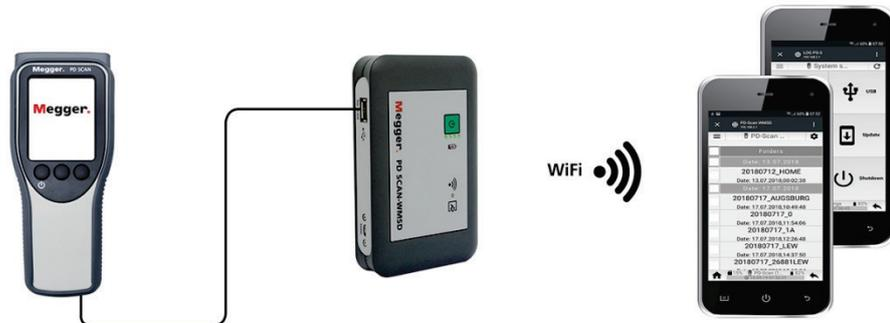
When a PD scan PD Scan is connected to the WMSD, all new measurement data sets are automatically downloaded to the internal memory of the WMSD. This function means that the mass storage device can also be used to collect the measurement data from multiple measuring devices that are in use without having to bring them to the office.
