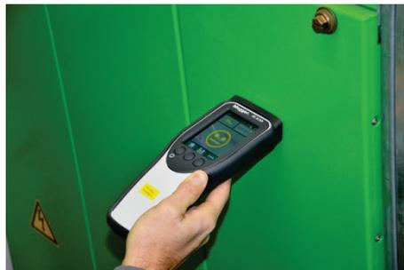
*Flexible airborne acoustic sensor* This external, acoustic sensor is specially designed for openings, air holes and gaps, out of which the acoustic waves of the partial discharges can escape from the switchgear.
