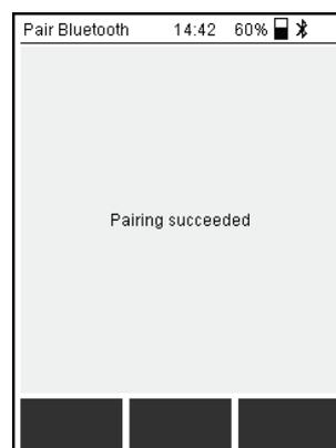
After being successfully paired for the first time, the headphones only have to be switched on after the PD Scan in future, and should then connect to it automatically. However, the
