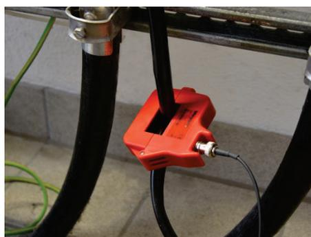
In principle, the PD Scan can also be used in combination with other HFCT couplers, as long as they feature an accessible BNC interface. However, depending on the sensor used, this may result in differences in the level display. The PD Scan has been precisely harmonised with the HFCT sensor in terms of its measurement accuracy.
