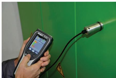
It is essential that this type of sensor is used correctly. The sensor head must be placed flush on a surface that is as smooth as possible. Even the smallest air inlets pose a risk of preventing signals caused by partial discharges from being measured.
