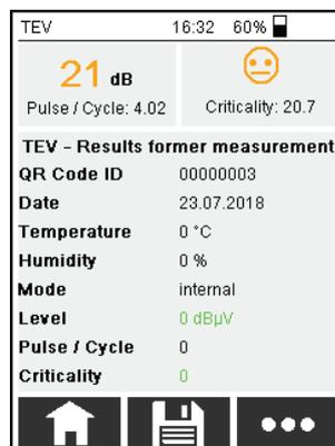
This screen allows you to quickly and reliably identify whether the measured values have, for example, worsened in comparison to a measurement performed 6 months ago.
