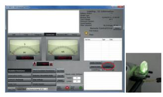
To activate the Import/Live Stream Control application click the Import soft button (circled) in the remote control application
