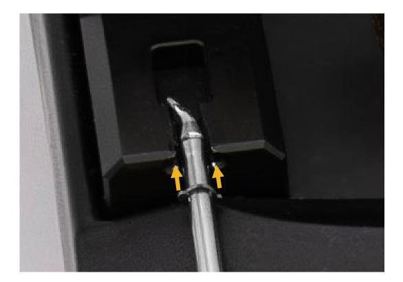
With the tip securely in the alignment tool, rotate the tweezer slowly in the required direction until the tip is in the desired position.
