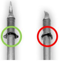
When horizontal, the wings of the alignment ring will match the opening of the alignment tool on the front of the workstand.
