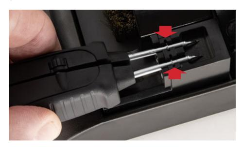
Carefully pull the tweezer backward, leaving cartridges safely in the removal tool. You may need to steady the workstand with your other hand.
