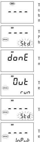
This screen appears each time the meter enters pump or pH calibration mode by pressing the **CAL** button. The meter is ready to start pump calibration by pressing the **PUMP** button. The meter returns to the main screen by pressing the **CAL** button.
