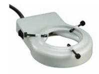
Fluorescent Ring Light provides full illumination with a powerful 17-watt, 5600°K lamp. A durable powder-coated metal housing protects the fluorescent lamp which has a rated lamp-life of 4,500 hours and produces 2,000 footcandles at 4.5" working distance.. Plug-in ballast with polarized plug is included.
