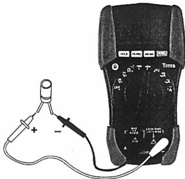
Fig. 8: Operation for Capacitance measurement
