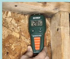
Measures % of Moisture in sheet rock and other building materials using direct pin method
