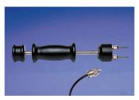
Two insulated pins with 1  $^{1}/_{16}$ " penetration. Used to measure wood moisture content at various depths.
