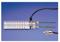
Two insulated pins with 3 1/4" penetration. Used for roofs, insulation, or EIFS.
