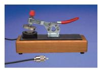
Clamp type for testing thin sheet stock, veneer, and fiberboard between two smooth disks.
