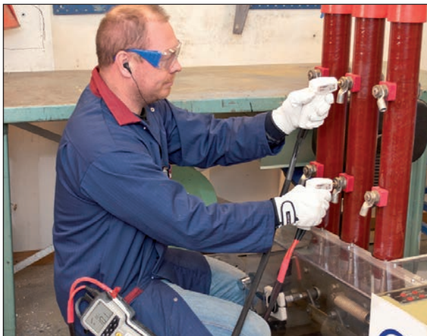
Hold probes / attach Kelvin clamps to CB and press trig / TEST button. A signal indicates whether test was pass or fail and result is logged in unit for later dump to PC.
