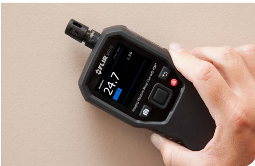
Verify moisture with Pinless measurements
