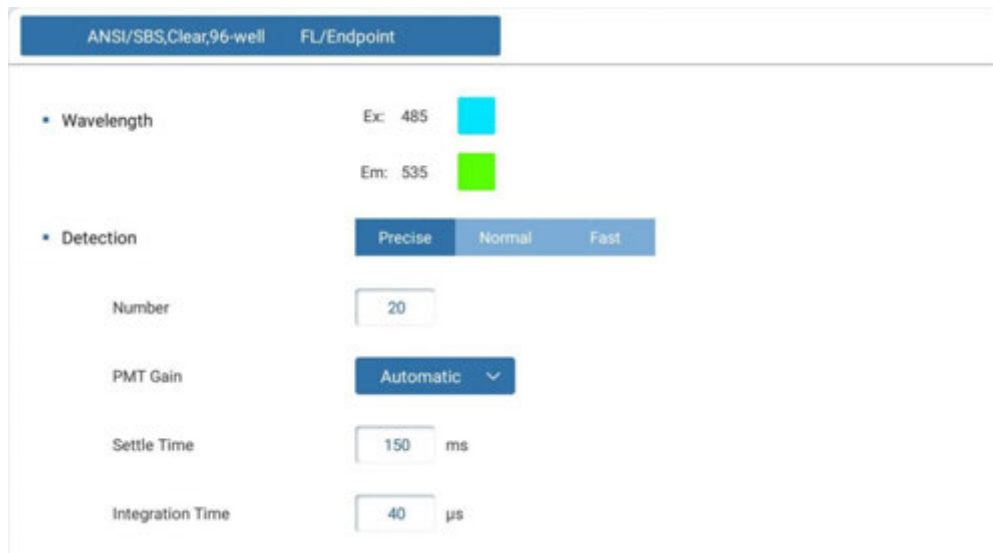
Figure 5.32.01 Step Settings Interface (Endpoint / Kinetic): Fluorescence
