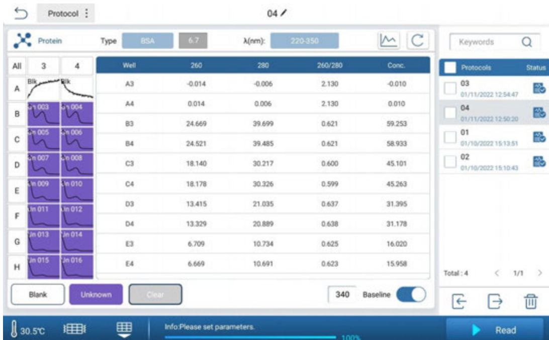
Figure 5. 52.02 Main Menu Interface : Proteins (Spectral)
