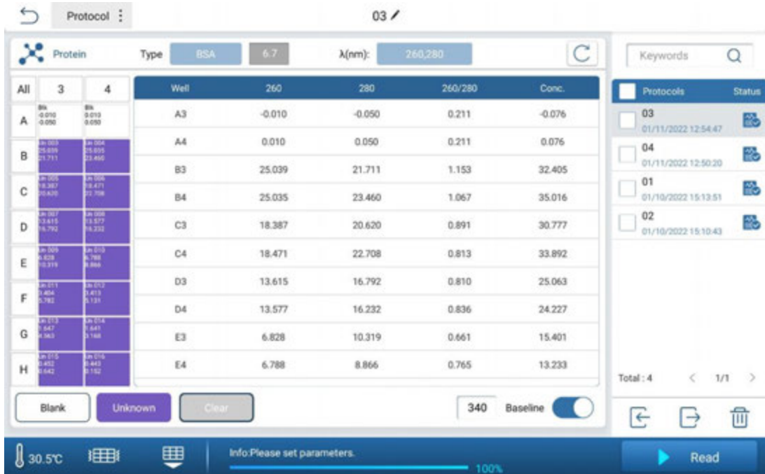
Figure 5.52.01 Main Menu Interface : Proteins (Fixed Wavelengths)
