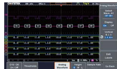
Display analog waveform converted from digital signal
