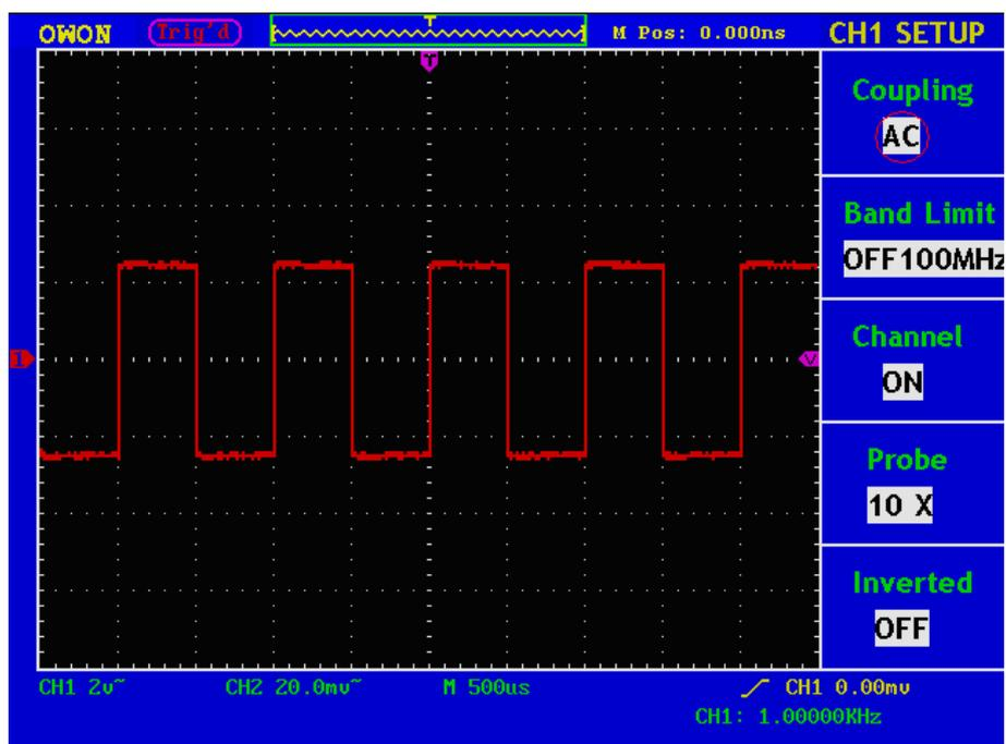
Fig. 5-2 AC Coupling Oscillogram
