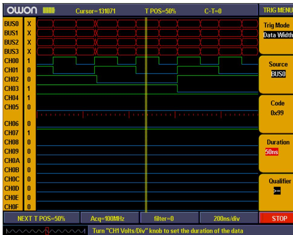
**Fig.5-65:** Data width trigger
