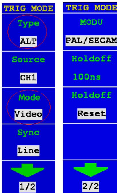
Fig.5-24 Alternate trigger(Trigger Type: video) Menu
