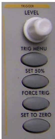
**Fig.4-11** Trigger Control Zone
