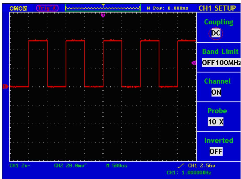
Fig. 5-3 DC Coupling Oscillogram
