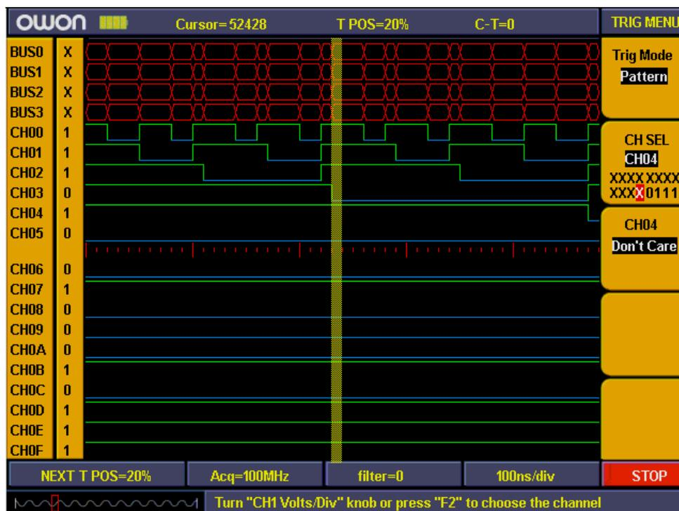
Fig.5-59: Pattern trigger
