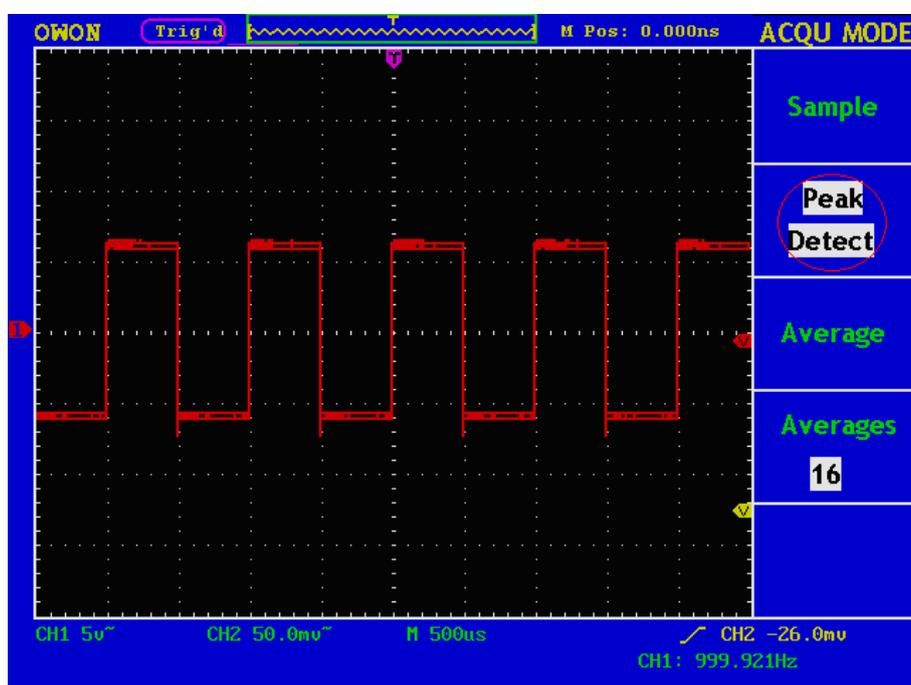
**Fig.6-4** Wave Form of the Signal Containing Noises
