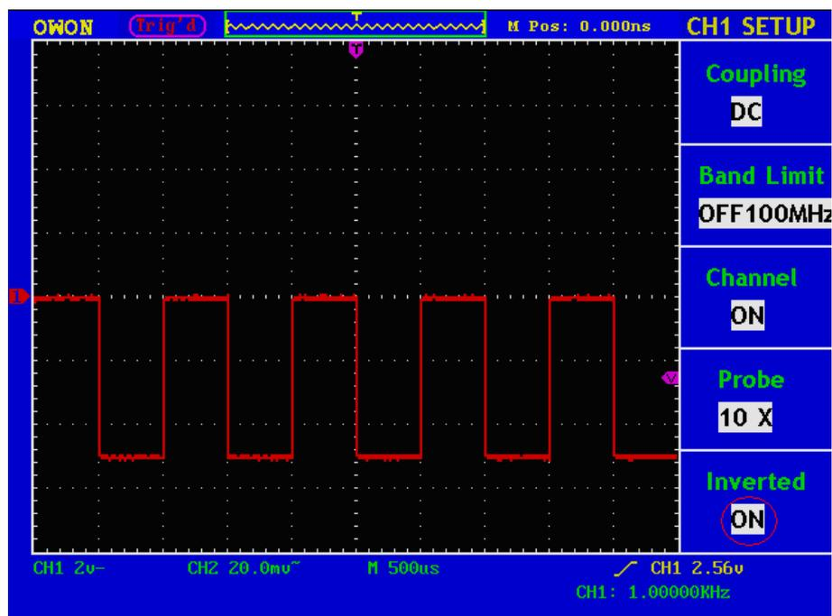
Fig. 5-7 Wave Form Inverted
