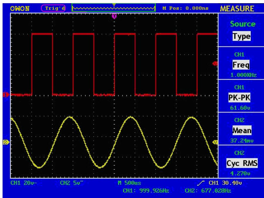
**Fig.5-44** Automatic Measurement
