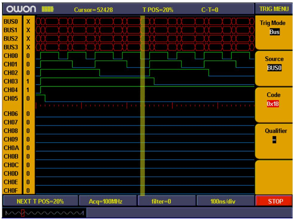
Fig.5-57: Bus trigger
