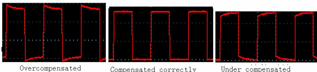
**Fig. 4-5** Displayed Wave Forms of the Probe Compensation
