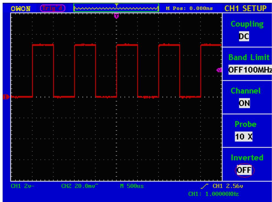
Fig. 5-6 Wave Form not inverted
