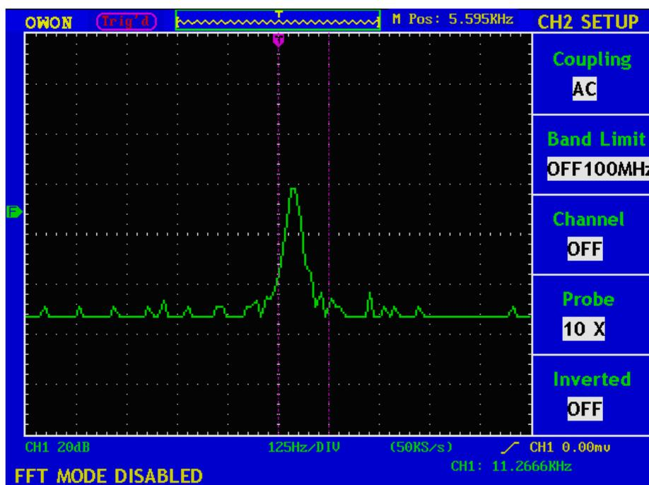
Fig. 5-4 Channel CH1 is disable under FFT mode
