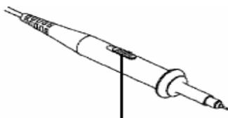
**Fig.4-7** Attenuation Switch
