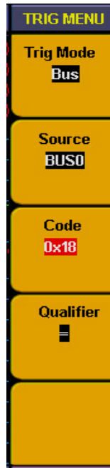
Fig.5-56: Bus trigger menu
