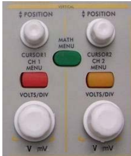
Fig. 4-9 Vertical Control Zone
