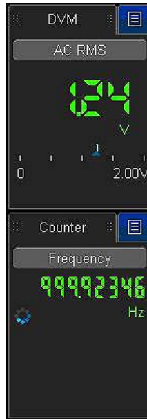
Figure 26. DVM and counter takes advantage of separate signal paths to provide measurements without a trigger, while still using the scope probes.
