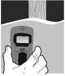
If the beeper fails to stop sounding as you move the instrument, there is something distorting the field behind the area that you have chosen. Release the **PUSH** button, choose another area, and repeat this step until you have successfully calibrated the MSV100 to the thickness of the surface.
