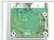
Double-sided glass epoxy PCB features fuse and diode Protection
