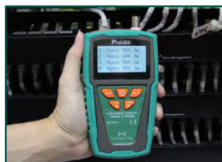
Locate break point and length measurement
