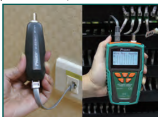
Verify LAN/ Telephone / Coaxial cable condition
