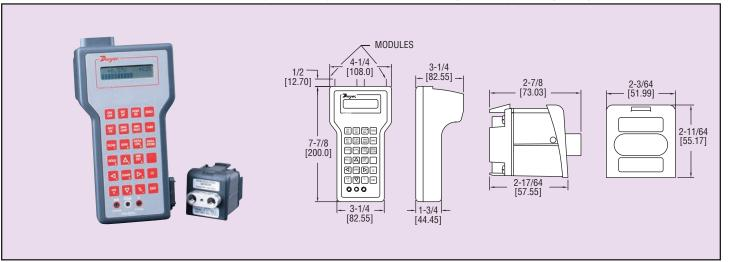
Series MC Portable Multi-Cal Pressure Calibrator performs a wide variety of simple and complex pressure based measurement, test, and calibration operations. Modular sensor design allows user to select pressure measurement range for application flexibility. Calibrator can accommodate up to two interchangeable pressure modules (sold separately below) in any combination of range or accuracy.
