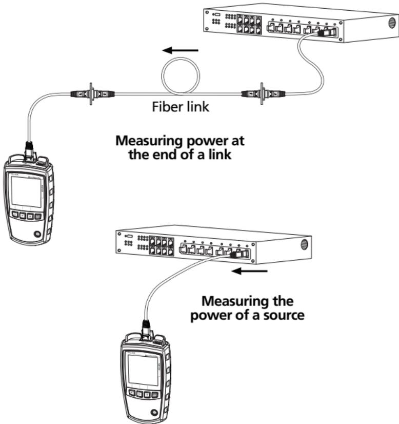
**Connections for Power Measurements**
