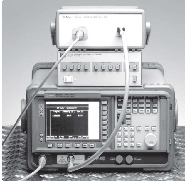
Figure 1. Noise source test system that includes the N2002A noise source test set, N8975A NFA and 11713A attenuator/switch unit
