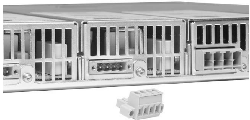
Figure 5. Quick disconnects for power and sense leads
