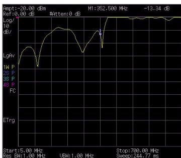
Figure 4-21 Measuring the Return Loss of the Filter
