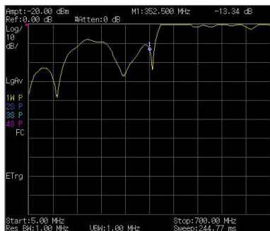
Figure 23 Measuring the Return Loss of the Filter
