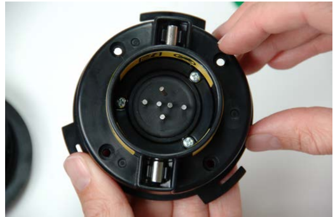
Figure 7 – Broken Contact Pin
