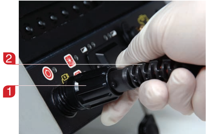
Figure 13 – Connecting to a SeeSnake CCU
