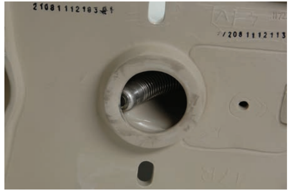
Figure 17 – Camera Head Blocked in Turn
