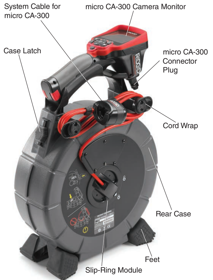
Figure 3 – Rear View (with the micro CA-300 inspection camera)
