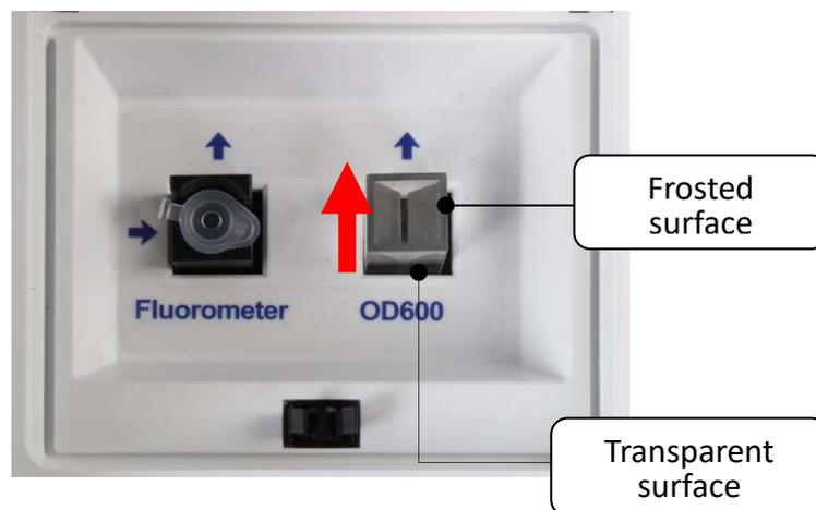
**Fig. 7 OD600 & Fluorometer Port**
