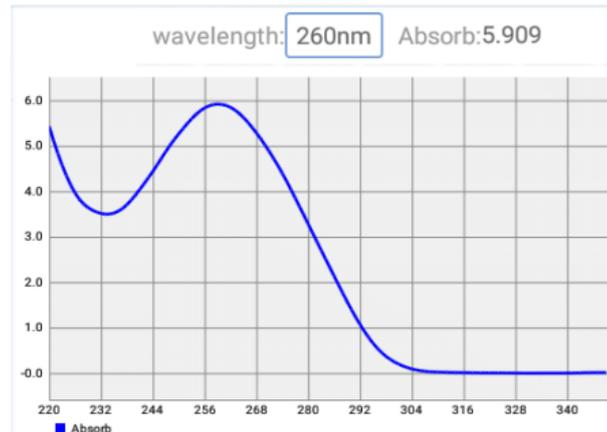
**Fig. 13 Nucleic Acid Sample Absorbance Curve (220nm – 350nm)**
