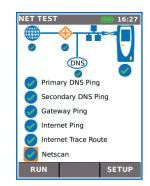
View network illustration to verify test results of each network component.
