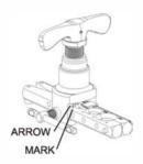
Turn the flaring drive handle clockwise until the clutch disengages automatically.
