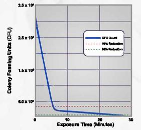
Adjustable pipetize were inoculated with S. sureus and placed in the UV Pipetiz Carousel. Individual pipetize were removed during the Auto-Decon<sup>™</sup> cycle at various intervals and rinsed to collect any residual contemination. The rinses were then plated and the CFU counted to determine the affectiveness of a single decontemination cycle.
