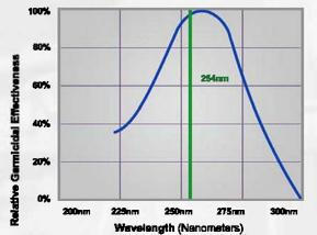
The blue curve, above, shows the germit.tiel effectiveness of UV light on E. Coll. The green line represents the 254 nm wavelength of industry standard germiddal lamps like the one at the core of the nUVAClean's pipets chember. This tamp emits greens than 80% of its light at 254 nm, which causes demage to the DNA of microorganisms, preventing their growth and reproduction, ultimately destroying them (see Figure 1.).
