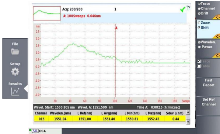
Fig. 19 Example of drift measurement, figure shows wavelength drift over time
