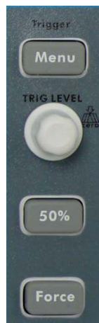
Figure 13. Trigger Control Zone.
