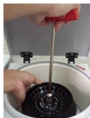
Tool for rotor with nut
