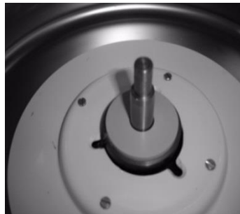
Motor shaft and chamber
