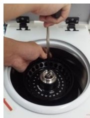
Tool for rotor without nut
