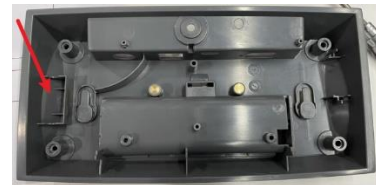
Fix the ferrite core on housing
