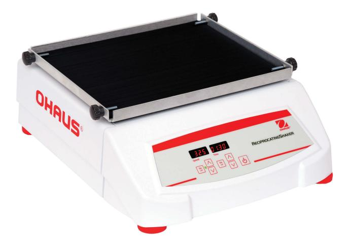
OHAUS Reciprocating Shakers are designed for a range of applications including cell cultures and extraction procedures that require accurate, repeatable results. Our shakers are microprocessor-controlled to provide consistent, uniform shaking action. The back-and-forth reciprocating motion has a 19 mm stroke length. Permanently lubricated ball bearings & maintenance-free, brushless DC motor provide reliable service and continuous duty operation.
