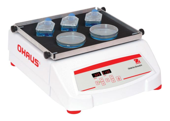
With load capacities from 35 to 150 lb and over 70 accessory options, OHAUS Heavy Duty Shakers are designed to handle a range of applications. Available as analog or digital models with microprocessor control to provide variable speed and consistent shaking, while ramping to the set speed. Microprocessor displays the last set-point and will restart if power is interrupted. Built-in tray and non-slip rubber mat included with all models.
