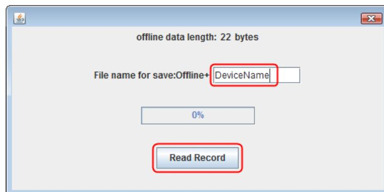
(6) Click "**Read Record**", the software will read the measuring data and save as a CSV file into computer. After reading, the dialog is as below:
