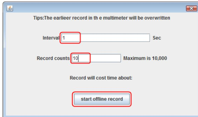
(3) Set "Interval" and "Record counts" (maximum records count is 10,000). Click "**start offline record**". The memory in the multimeter can only store the recording data of one time. When start to record, the earlier offline record stored in the multimeter will be overwritten.
