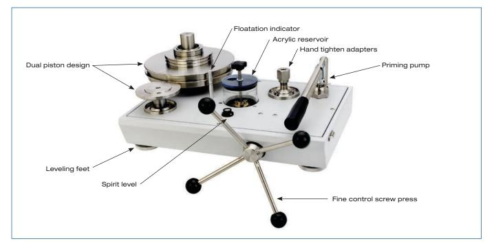
2 Fluke Calibration P3000 Series Hydraulic Deadweight Testers Models P3100 and P3200
