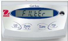
To help adapt the balance to real life working conditions, the PAJ is designed with selectable environmental settings. When working in harsh environments, the balance can be adjusted to compensate for vibrations and other disturbances. Conversely, the balance can be adjusted for working in slow filling applications where sensitivity is a must.
