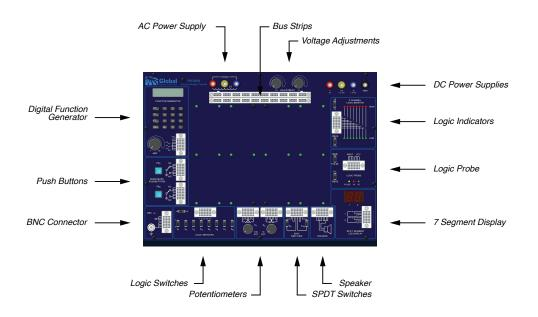
Figure 1 PB-505A Components
