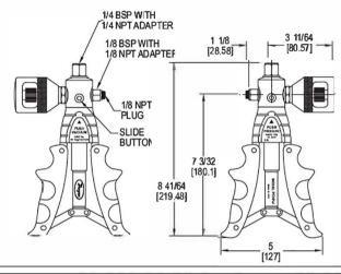
The **SERIES PCHP** Pneumatic Calibration Hand Pump sources pressure and vacuum to check calibration of gages, switches, transmitters, and recorders. The contoured cushion handles provide extra comfort while preven ing the pump from sliding.
