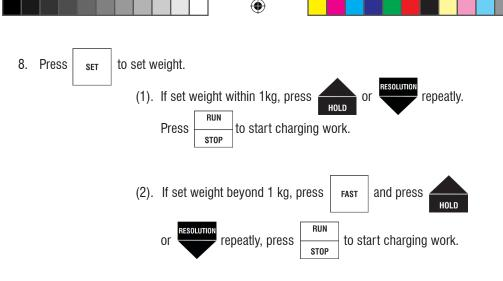
9. When finished refrigerant charging, the Valve will auto shut off and alarm for 6 seconds.
