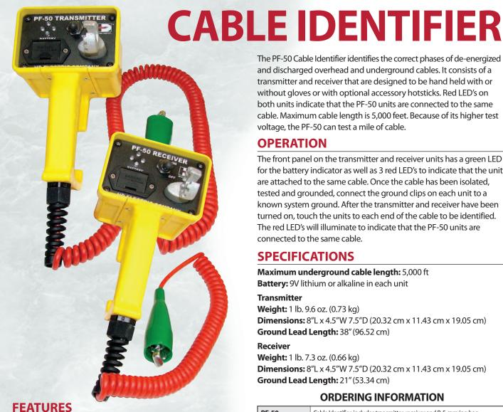
The PF-50 Cable Identifier identifies the correct phases of de-energized and discharged overhead and underground cables. It consists of a transmitter and receiver that are designed to be hand held with or without gloves or with optional accessory hotsticks. Red LED's on both units indicate that the PF-50 units are connected to the same cable. Maximum cable length is 5,000 feet. Because of its higher test voltage, the PF-50 can test a mile of cable.
