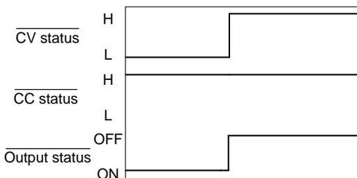
**CC MODE:** The diagram below shows the timing diagram when the output is turned on when the PFR-100 is set to CC mode.
