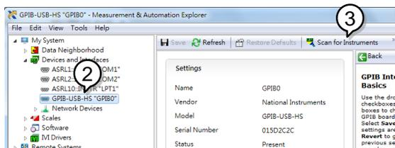
4. Select the device (GPIB address of PFR-100) that now appears in the *System>Devices and Interfaces > GPIB-USB-HS "GPIBX"* node.
