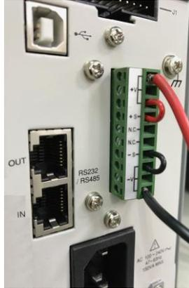
6. If using voltage sense, remove the sense terminal joining cables and connect sensing wires to the load(s).
