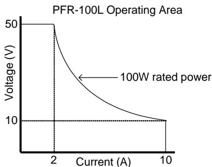
When the power supply is configured so that the total output (current x voltage output) is less than the rated power output, the power supply functions as a typical constant current,
