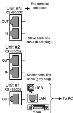
5. Terminate the OUT port of the last unit with the end terminal connector included in the PSU-232 or PSU-485 connection kit.
