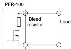
Bleed resistors are designed to dissipate the power from the power supply filter capacitors when power is turned off and the load is disconnected. Without a bleed resistor, power may remain charged on the filter capacitors for some time and be potentially hazardous.
