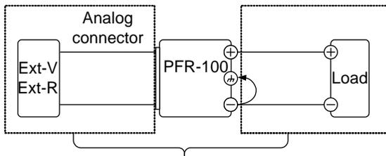
(-----) Insulation capacity  $\geq$  voltage of power supply with respect to ground
