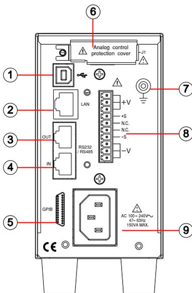
1. **USB**                    USB port for controlling the PFR-100 remotely.
