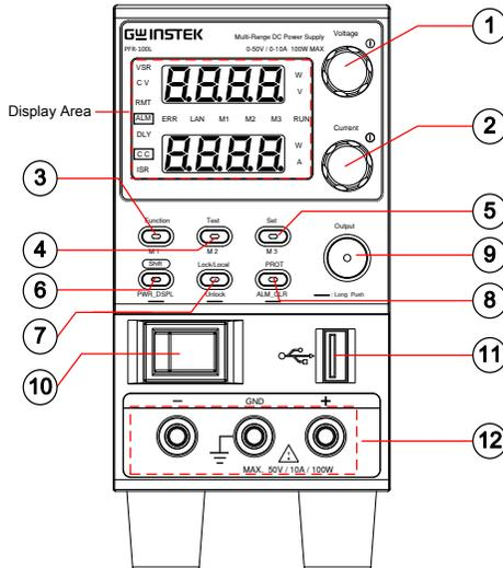
**Display Area** The display area shows setting values, output values and parameter settings. The function LEDs below show the current status and mode of the power supply. See page 16 for details.
