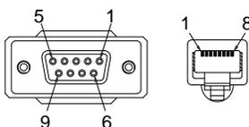
RS485 cable with DB9 & RJ-45 shielded connectors from PSU-485 connection kit
