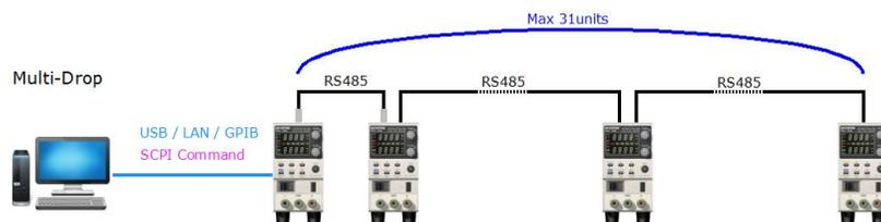
There is a mode for controlling multiple units. This mode allows the user to enter the SCPI commands developed for the instrument (Multi-Drop mode). In this mode, only the Multi-Drop parameters have to be specified. Each unit is assigned a unique address and can then be individually controlled from the host PC.
