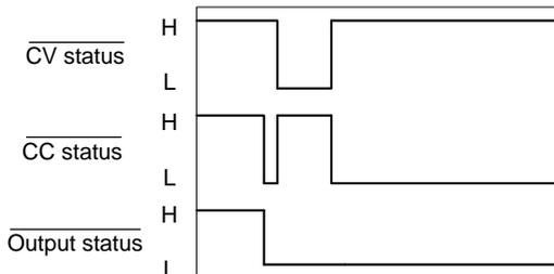
**CC MODE:** The diagram below shows the output status lines when the output is turned off in CC mode.
