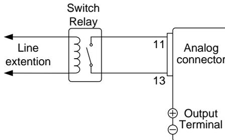
If a single switch control is to be used for multiple units, please isolate each instrument. This can be achieved by using a relay.
